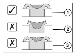
Fig. 5-69: Checking the riveting
