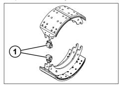
Fig. 5-72: Inserting the cam rollers
