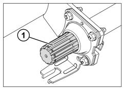
Fig. 5-32: Preparing the brake camshaft
