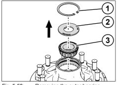
Fig. 5-52: Removing the outer bearing
