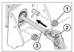
Fig. 5-20: Inserting the brake cylinder
