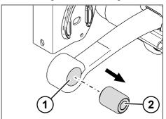
Fig. 5-123: Removing the silent bearing
