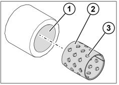
Fig. 5-70: Inserting the cam roller bushing
