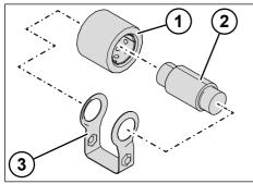
Fig. 5-71: Fitting the cam roller
