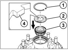
Fig. 5-58: Inserting the outer bearing
