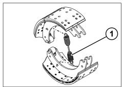
Fig. 5-61: Unhooking the release spring
