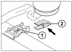
Fig. 5-108: Fastening the shim
