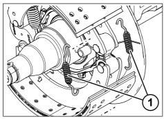
Fig. 5-59: Unhooking the fixed-point springs
