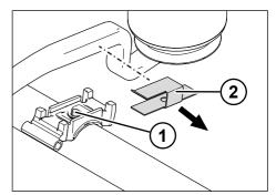
Fig. 5-107: Removing the shim
