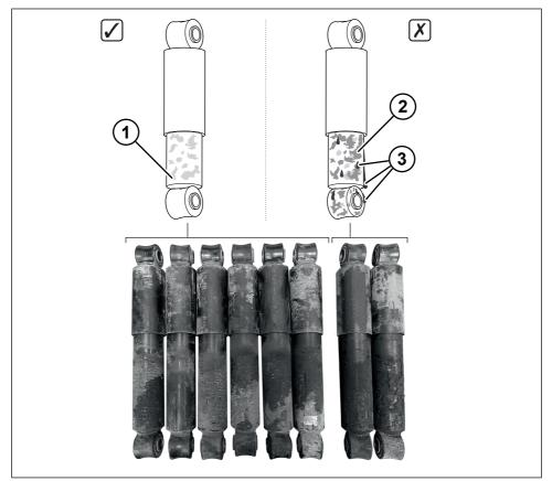
*Fig. 4-6:* Examples of shock absorber defects Perform the following maintenance work:
