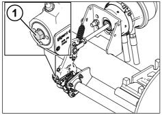
*Fig. 5-10:* Loosening the setting nut of the ASA
