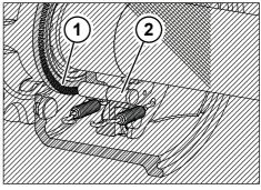
*Fig. 5-50:* Sectional view of the ABS magnet wheel
