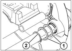
Fig. 5-79: Securing the circlip
