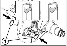
Fig. 5-88: Inserting the sealing rings
