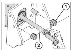
Fig. 5-12: Removing the brake cylinder
