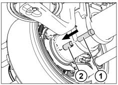
Fig. 5-49: Fastening the ABS sensor
