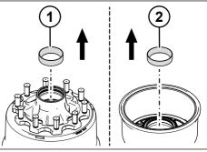
Fig. 5-54: Removing the bearing rings
