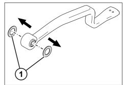
Fig. 5-116: Removing the thrust washers
