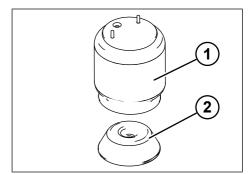
*Fig.* 3-12: Air spring bellow rail loading components
