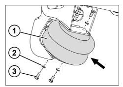
Fig. 5-101: Fitting the two-fold bellow
