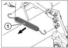
Fig. 5-27: Unhooking the tension spring
