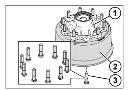
Fig. 5-44: Removing the brake drum
