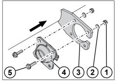
Fig. 5-84: Fitting the spherical cam bearing
