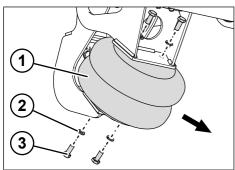
Fig. 5-100: Removing the two-fold bellow
