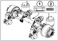
*Fig. 1-1:* Type plate position
