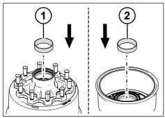
Fig. 5-56: Inserting the bearing rings
