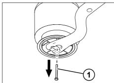
*Fig. 5-114:* Removing the fitting of the air spring bellow
