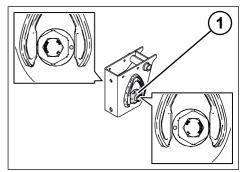
Fig. 5-129: Adjusting the eccentric nuts identically
