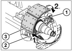
*Fig.* 5-63: Inserting the upper brake pad carrier
