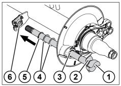
Fig. 5-78: Inserting the brake camshaft
