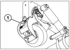
Fig. 5-99: Removing the compressed air line
