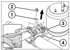
Fig. 5-106: Loosening the retainer nuts
