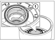
Fig. 5-55: Cleaning the bearing seats
