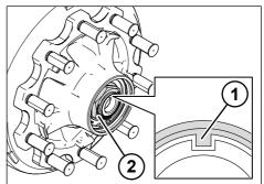
Fig. 5-39: Removing the axle nut
