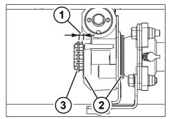
Fig. 5-34: Inserting the circlip
