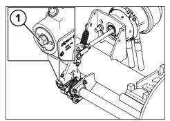
*Fig. 5-38:* Tightening up the setting nut on the ASA
