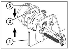
Fig. 5-24: Inserting the emergency release screw
