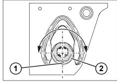
*Fig. 5-120:* Adjusting the play of the air spring link
