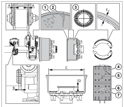
Fig. 4-5: Wear dimensions: Air suspension, brakes and ASA
