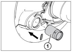
*Fig. 5-87:* Inserting the brake carrier cam bearing bushing
