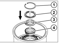
Fig. 5-57: Inserting the inner bearing
