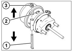
*Fig. 5-16:* Removing the emergency release screw
