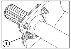
*Fig. 5-81:* Greasing the spherical cam bearing
