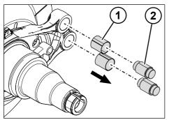
Fig. 5-73: Removing the fixed-point bearing
