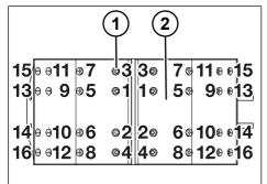
Fig. 5-68: Riveting sequence
