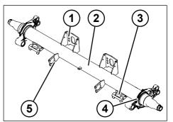
Fig. 3-2: Axle body components (bottom air spring link)
