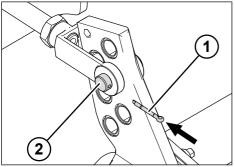
Fig. 5-21: Inserting the fork head bolt
