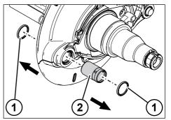
Fig. 5-86: Removing the brake carrier cam bearing bushing
