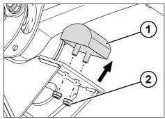
Fig. 5-103: Removing the wear block
