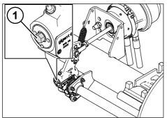
*Fig. 5-28:* Loosening the setting nut of the ASA
