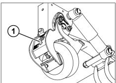
Fig. 5-102: Fastening the compressed air line
