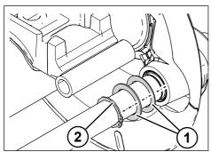
Fig. 5-76: Loosening the circlip
