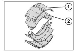
Fig. 5-66: Removing the brake pad
