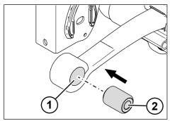
Fig. 5-124: Inserting the silent bearing
