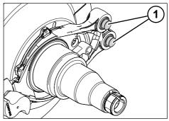
Fig. 5-75: Greasing the brake pad carrier contact surface
