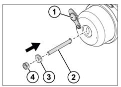
Fig. 5-17: Inserting the emergency release screw
