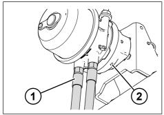
Fig. 5-25: Fastening the compressed air lines
