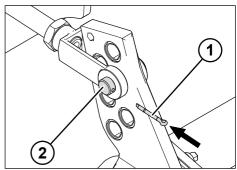
Fig. 5-35: Inserting the split pin
