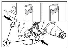
Fig. 5-90: Inserting the sealing rings
