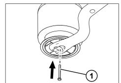
*Fig. 5-119:* Fastening the air spring bellow fitting
