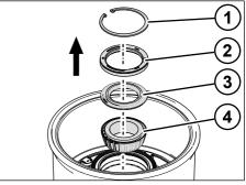
Fig. 5-53: Removing the inner bearing
