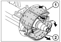
Fig. 5-60: Removing the brake pad assembly
