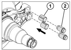
Fig. 5-74: Inserting the fixed-point bearing
