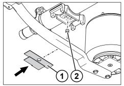
Fig. 5-112: Fastening the shim
