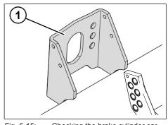
Fig. 5-15: Checking the brake cylinder carrier
