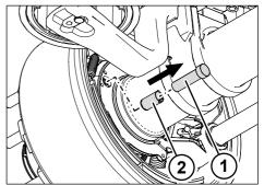
Fig. 5-48: Removing the ABS sensor
