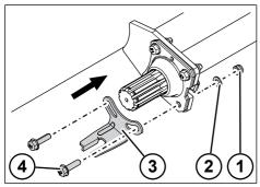
Fig. 5-85: Inserting the ASA fixed-point tab
