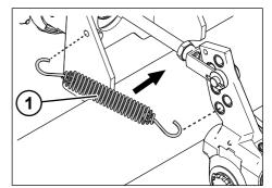
Fig. 5-22: Mount the tension spring
