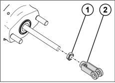
Fig. 5-14: Removing the fork head
