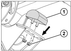
Fig. 5-104: Fitting the wear block
