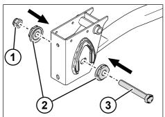
Fig. 5-118: Fastening the link fitting
