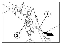
Fig. 5-11: Removing the fork head bolt
