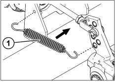
Fig. 5-36: Mount the tension spring
