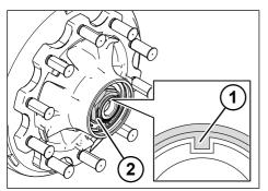
Fig. 5-43: Inserting the axle nut
