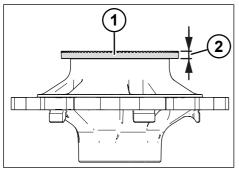
*Fig. 5-51:* Checking the parallelism of the ABS magnet wheel
