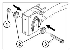
Fig. 5-126: Fastening the link fitting
