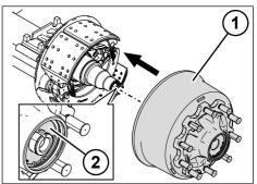
Fig. 5-42: Brake drum and hub unit
