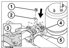
Fig. 5-109: Fastening the retainer nuts
