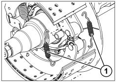
Fig. 5-65: Attaching fixed-point springs
