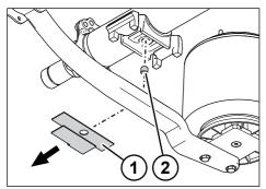
Fig. 5-111: Removing the shim
