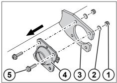
*Fig. 5-83:* Removing the spherical cam bearing
