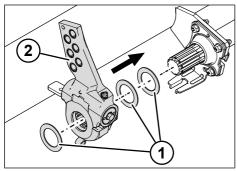
Fig. 5-33: Inserting the ASA and spacer washers
