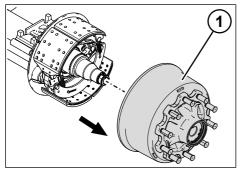
*Fig. 5-40:* Removing the brake drum and hub unit
