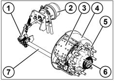
Fig. 3-13: Brake components
