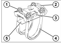
Fig. 3-3: Integration components (top air spring link)
