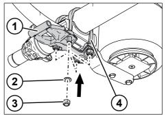
Fig. 5-113: Fastening the retainer nuts
