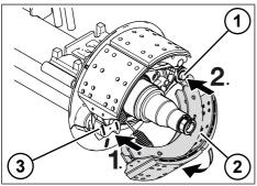
Fig. 5-64: Inserting the lower brake pad carrier
