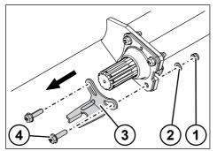
Fig. 5-82: Removing the ASA fixed-point tab
