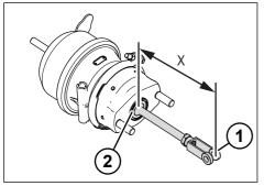
Fig. 5-13: Distance measurement
