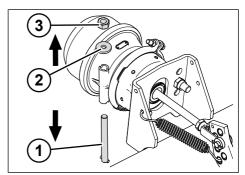
*Fig. 5-7:* Removing the emergency release screw
