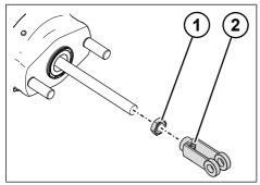
Fig. 5-18: Inserting the fork head
