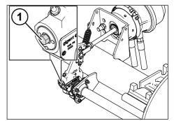
Fig. 5-26: Tightening up the setting nut on the ASA
