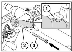
Fig. 5-93: Inserting the shock absorber
