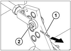
Fig. 5-29: Removing the fork head bolt
