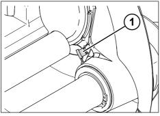
*Fig. 5-80:* Greasing the brake carrier cam bearing bushing
