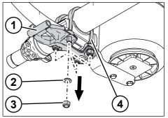
*Fig. 5-110:* Loosen the retainer nuts [integration, bottom air spring link]
