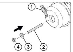
Fig. 5-8: Install the emergency release screw
