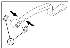
Fig. 5-125: Fastening the thrust washers
