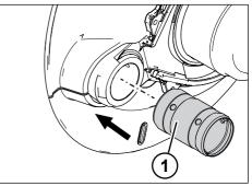
*Fig. 5-89:* Inserting the brake carrier cam bearing bushing
