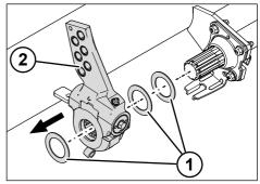
Fig. 5-31: Removing the ASA
